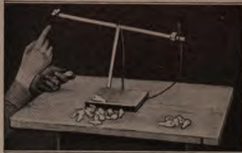
Perfect Aluminum Castings are Distinguished from Those Having Air Holes by Testing for Weight with a Special Balance
